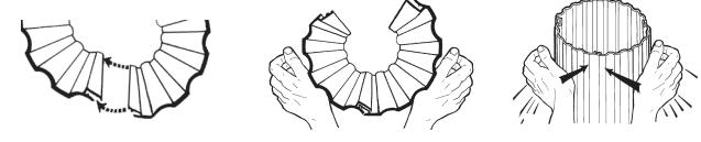
**(10" & 12" Columns)** Hinge small hooked ends into large hooked ends until one stave remains. Slide the final stave in place, tapping gently with a rubber mallet until ends align.
