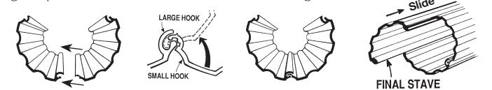
**(15", 18", 24", and 30" Columns)** Slide ALL staves together, pairing small hooked ends with large hooked ends. Gently tap with rubber mallet until ends align.
