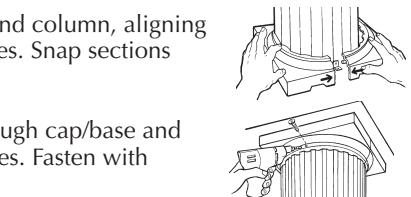
**STEP 2:** Drill two holes through cap/base and into column on opposite sides. Fasten with screws provided.
