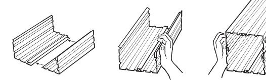
**(Smooth and Panel Columns)** (A) Fit two staves together, tongue into groove. Tap with heel of hand or rubber mallet until staves snap together. (B) Repeat with remaining two staves to create half sections. (C) Fit half column sections together, tongues into grooves, and snap to form a full column.
