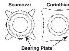
**Note:** If using Scamozzi or Corinthian caps, staves will stop at bearing plate welded to the top surface of caps.
