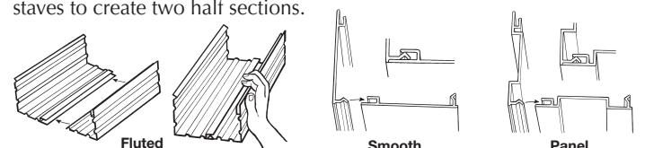
**Note:** Panel columns in wrap-around applications require Panel Column Trim Inserts. Visit [superioraluminum.com/technical-information/assembly-instructions/](http://superioraluminum.com/technical-information/assembly-instructions/) for installation instructions.
